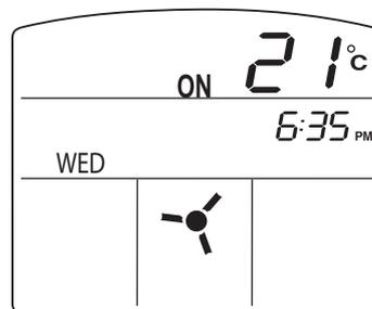
Fan-only display with zones 1, 2 and 3 on - single SCC with zones, or multiple SCC system.
