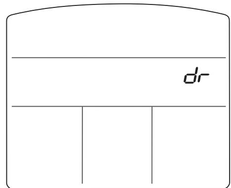
During the drain operation all buttons are in-operative. When the cooler is re-started, there will be a delay while the cooler tank is re-filled with fresh water.
